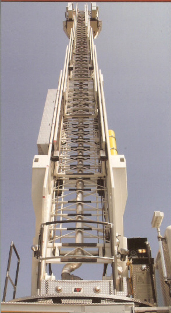
Clear ladder walkway for easier access
