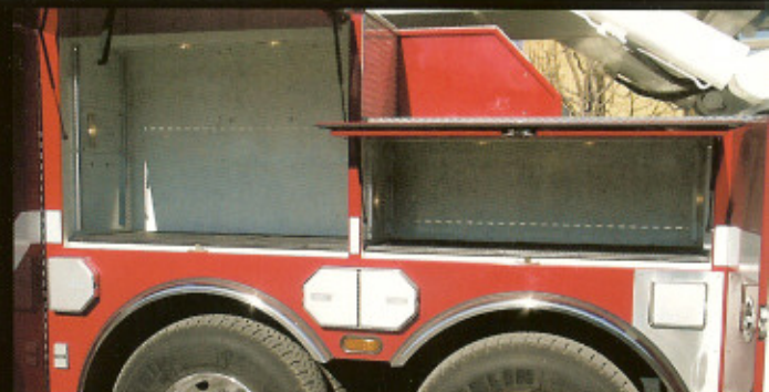
Full-height and full-depth body compartments with up to 25" depth
