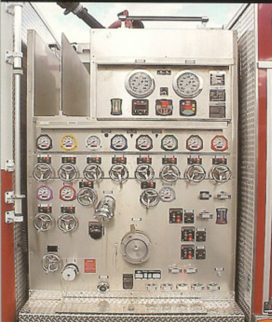
Brushed stainless steel pump module resists "rust" or "white" corrosion
