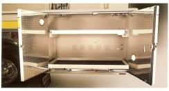
MARION'S EXTRUDED DOORS interlock for superior strength. They're flush mounted for snag-free performance. The door pans are made of aluminum diamond plate and are easily removable for servicing the locks. On the job, a glueless, watertight seal keeps weather out and your equipment dry.
